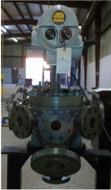
A single MSV can manifold as many as seven flow lines through it simultaneously. Multiport Selector Valve (MSV) allows the diversion of fluids from a single flow line to a test outlet or a sampling device
